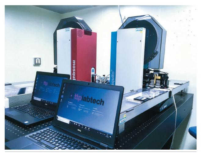
Figure: An overview of the high-throughput single-cell RNA sequencing platform. Two nanoliter liquid handling robots are shown.
